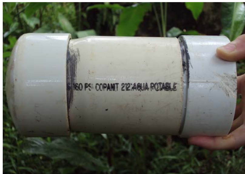
Figure 30. Current chlorination tablet holder used in Quebrada Caracol community
