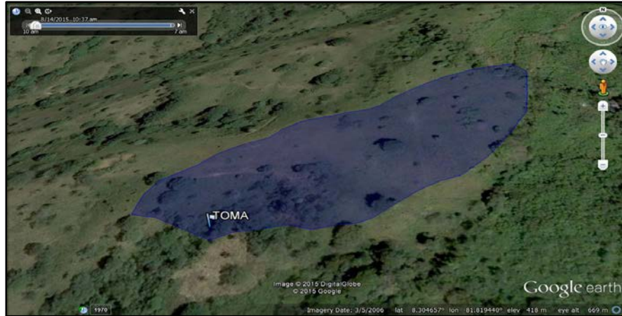
Figure 6: Area of Watershed Found Using Google Earth Polygon Feature
